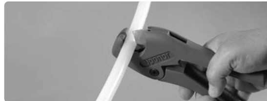
Figure 3-4: Square-cut the PEX Tubing
