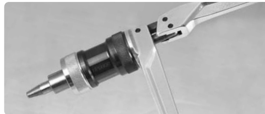
Figure 3-3: Operate Expander Tool to Rotate Adapter
