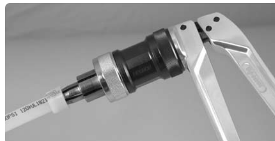
Figure 3-6: Insert Expander Head into Tubing
